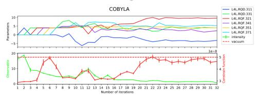
Vacuum readings before chopper dump as BLMs  $\rightarrow$  constraint for minimising pulse shape error while adjusting 6 quadrupoles
