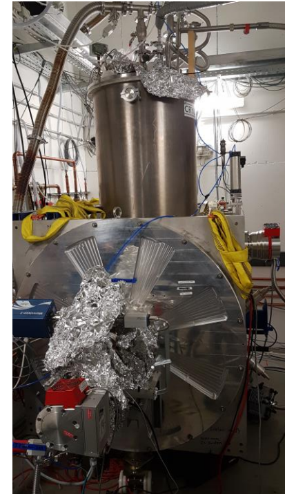
Test cryostat with superconducting cavity at test bunker
