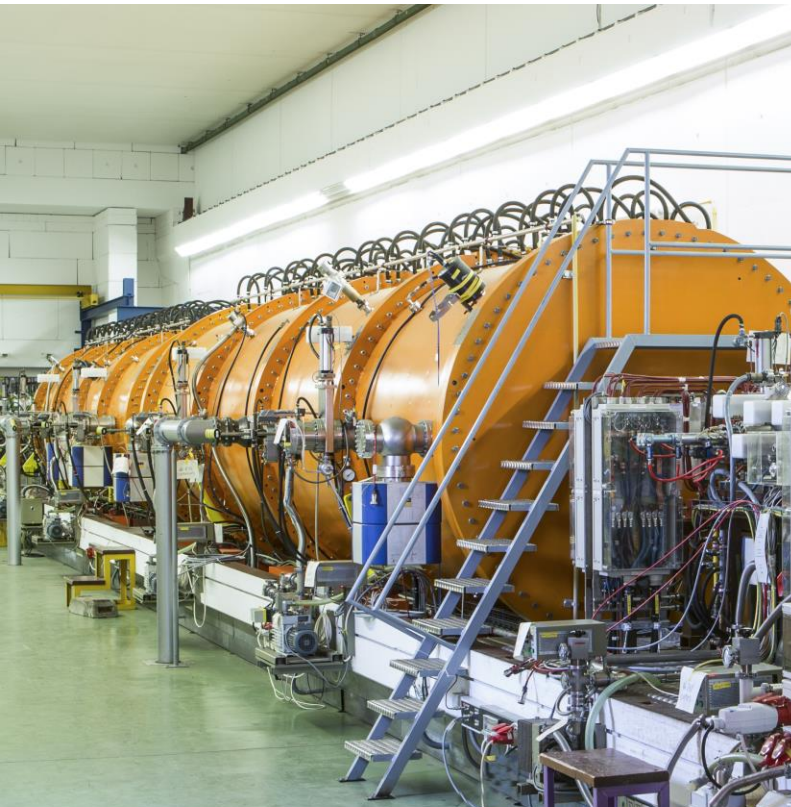
GSI 91 MV High Current Linac, 36 MHz
