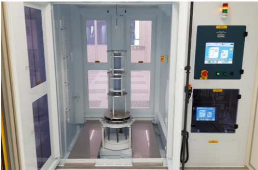
High Pressure Rinsing at clean room
