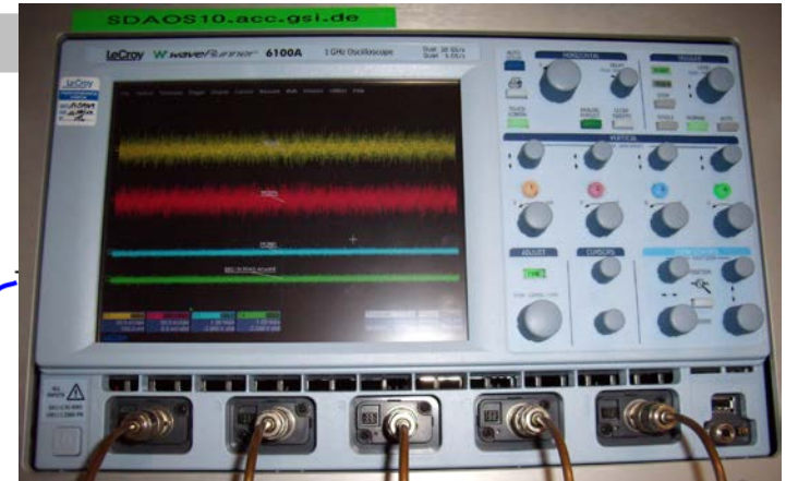
CNAO RFQ ToF with phase probes
