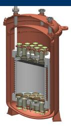
DarkSide-20k: 20 t (fiducial) at Gran Sasso, starting in 2027 DarkSide-LowMass: 1 t (fiducial), S2 only to lower threshold  $\rightarrow$  more ultrapure Ar needed P. Agnes et al, Phys. Rev. D 107 (2023) 112006 ARGO: ~360 t, at SNOLAB
