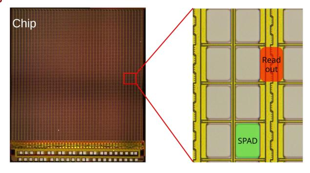
SPADs (single photon detector) and their CMOS readout electronics are manufactured on one silicon chip:
