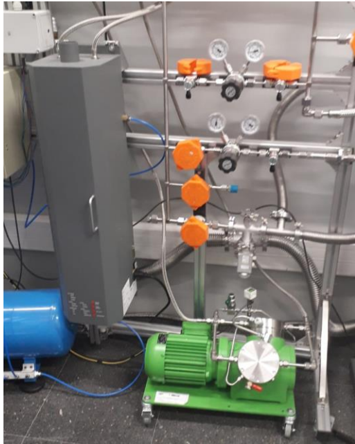
Hot getter from Sigma Technologies PS4 MT15 R2
