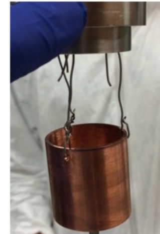
Figure 4. The inner copper crucible to hold the TPB powder is attached to a stainless steel top hat and lowered into the spherical source.
