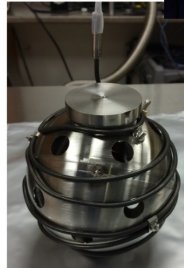
Figure 3. Final stainless steel TPB deposition source. The coil heater is held in thermal contact with the sphere with compressed tabs.
