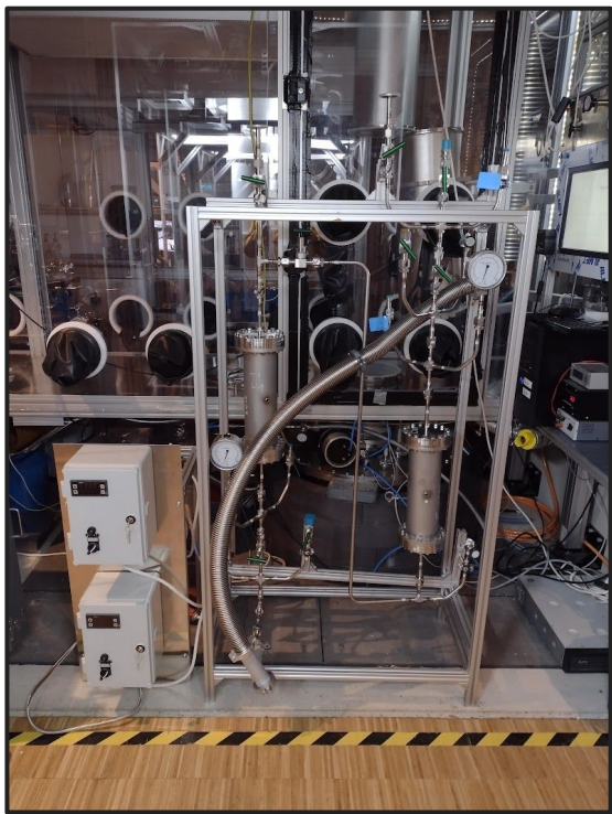
Purification setup w/o thermal insulation
