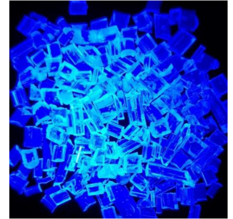
PEN granulate illuminated by UV light
