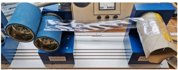
Small-scale film extruder at ipf Dresden
