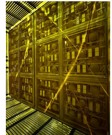
SBND PDS boxes behind anode wire planes
