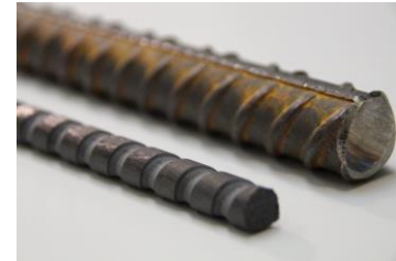
Comparison reinforcing carbon and steel (from https://www.carbocon.de )
