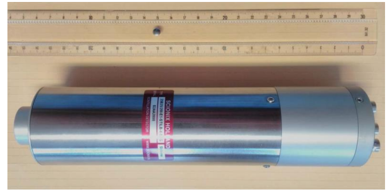
Stilbene detector, assembled by Scionix
