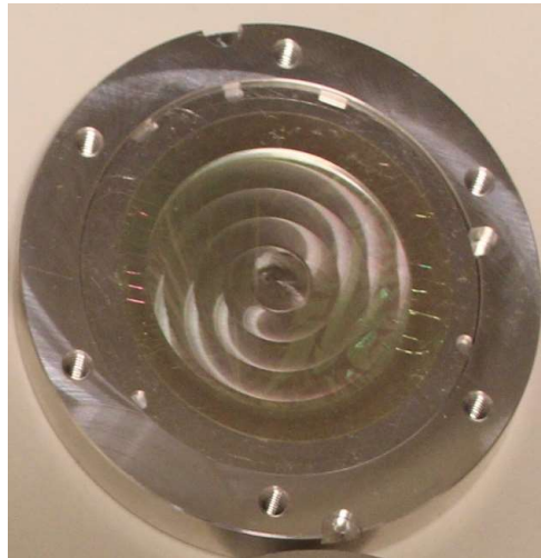
Polyimide foil Areal density: 60 \mu\text{g}/\text{cm}^2 In-situ polymerisation JRC-Geel
