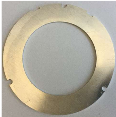
Al-ring 1mm thick \text{\O}_{\text{out}} 60mm \text{\O}_{\text{in}} 40mm CEA, JRC-Geel
