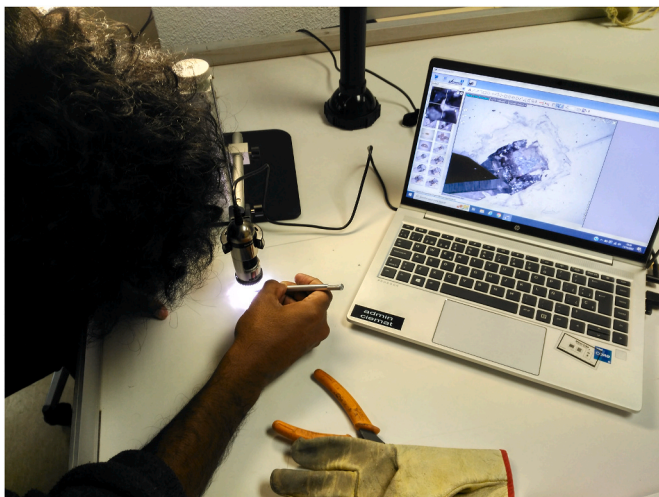
Fig. 13. An USB microscope connected to a PC is used for most of the repairing steps.
