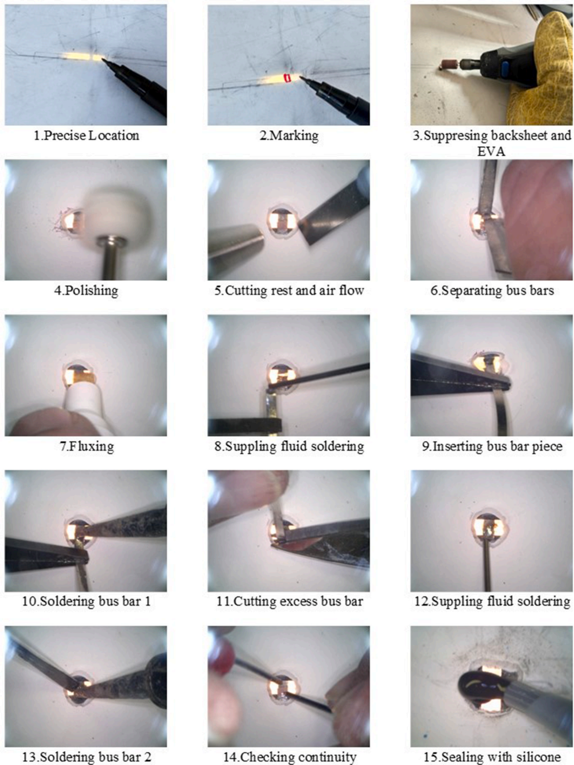
Fig. 14. Steps for repairing interrupted ribbon bus bar cell interconnection. For better illustration the sequence correspond to various ribbon bus bar repairs.
