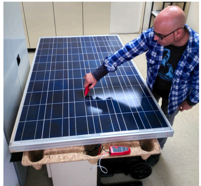
Fig. 4. Location of twin ribbon bus bar interruptions using tone tester and taking module frame as electrical earth. The module is isolated using pallet of chipboard between the work-table and the PV module. The operator displace the receiver sensor head following the ribbon bus bars, until finding a sound change which informs of a possible ribbon bus bar interruption.
