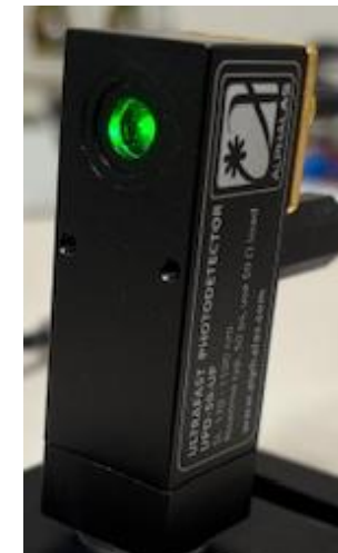
7 GHz VIS free-space photodetector
